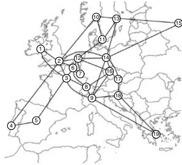
Fig. 8. European COST 239 Network (19 nodes, 37 bidirectional links)
